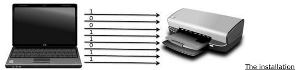
and troubleshooting is easier in parallel transmission system due to its placement in a single physical cable. Parallel Transmission uses a 25 pin port having 17 signal lines and 8 ground lines. The 17 signal lines are further divided as
