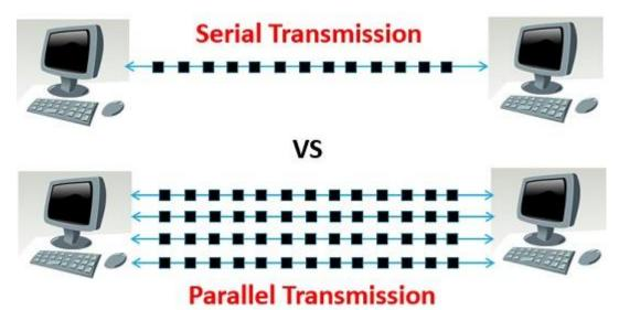
For transferring data between computers, laptops, two methods are used, namely, Serial Transmission and Parallel Transmission. There are some similarities and dissimilarities between them. One of the primary difference is that; in Serial Transmission, data is sent bit by bit whereas, in Parallel Transmission a byte (8 bits) or character is sent at a time.
